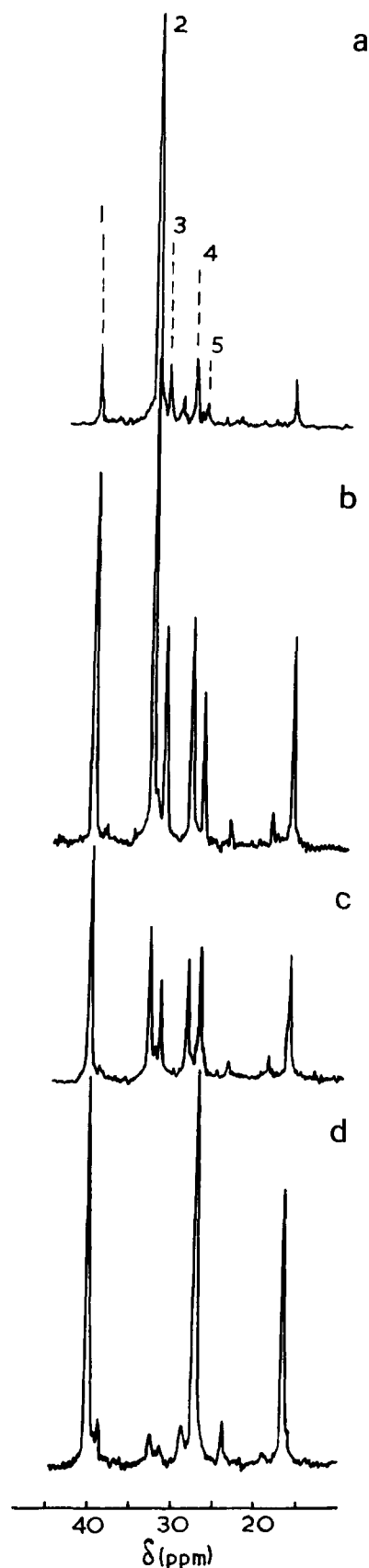
Figure 2 ^{13}\text{C} n.m.r. spectra of trans -1,4-copolymers of butadiene and isoprene: (a) 35 mol% isoprene; (b) 50 mol% isoprene; (c) 75 mol% isoprene and (d) polyisoprene synthesized in the presence of (\text{C}_4\text{D}_7\text{NiI})_2
